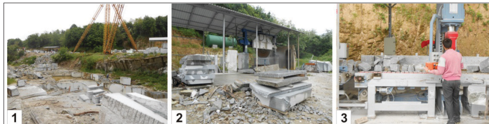
Figure 2 – “Babića Rt” quarry, 1. Exploitation of granite blocks; 2. Saw cutting of granite slabs; 3. Production of granitic cubes (photo: I. Carević)
