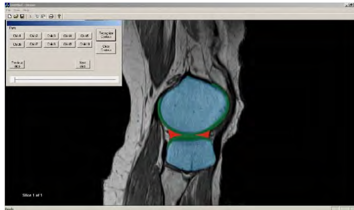
Fig. 4. Segmentation of the knee model from MRI slices. Sagittal view MRI of the left knee. The bone geometry, cartilages and meniscuses are digitized for 3D finite element model
