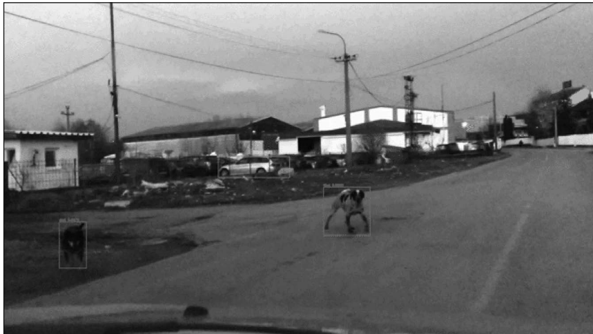
Figure 6. Detection of dogs on the road from the moving vehicle using YOLO
