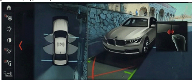
Figure 4. A bird's-eye view of the car and an outline of the car's environment with 360° rotation (DeMuro, 2018)
