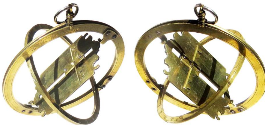
Fig. 1. The UERD of Professor Danić: the dial's face – the side with the latitude scale (left) and the back of the dial (right)
